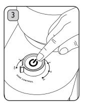
Plug in the Power Cord at the mains and press the Grind Button to start grinding. The Grinder will stop automatically when the selected dose has been dispensed. You can press the Grind Button at any time to manually stop grinding. NOTE: Do not grind past the 'MAX' indicator on the Grind Container to prevent overheating.
