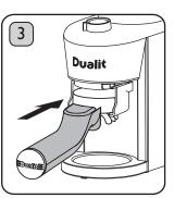
When using the Portafilter Cradle the Dose Control should be set to 2. For accurate dosing and less waste, weigh the amount of beans you need, add to the Bean Hopper, then grind through before tamping to the right level. As a guide, we recommend 7 - 10g for a single espresso and 14-20g for a double.
