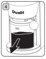
Remove the Grind Container. Tap to loosen grounds before decanting. NOTE: Unplug after use. **Risk of electric shock and fire.**
