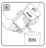
With the appliance unplugged and the Bean Hopper, Upper Burr, Grind Container/Portafilter Cradle removed, tip the Main Body over a bin. This will remove any remaining beans and grounds from the Lower Burr. Wipe down the Main Body of the machine with a damp, non-abrasive cloth. NOTE: Do not clean any Grinder parts or accessories in the dishwasher.
