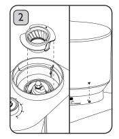
With the machine unplugged, check that the Upper Burr is located correctly. Check that there are no foreign bodies in the Hopper.
