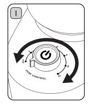
The Dose Control Dial is a rough guide for how many cups of coffee are required. Turn the dial so that the indicator aligns with the number of cups you wish to make. The amount of coffee dosed will change depending on the grind size setting. See page 10 for the Grind Chart.
