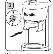
With the appliance unplugged, remove the Grind Container. Slide the Portafilter Cradle, as illustrated, under the Grind Outlet. Plug in the appliance and select a fine grind setting, see page 13 for Quick Start Grind Settings for guide.
