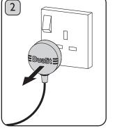
Ensure that the machine is unplugged and the Bean Hopper and Grind Container are empty of packaging material and coffee. Wash the Bean Hopper and Lid, Cradle, Grind Container, Container Lid and Cap in warm, soapy water then rinse and dry thoroughly before reassembling.
