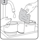
Remove the Grind Container and empty out any remaining coffee. Wash the Grind Container, Container Lid and Bean Hopper in warm, soapy water. Rinse, then dry thoroughly before storing.
