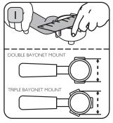
To check whether your portafilter will fit the Portafilter Cradle, measure the outer diameter of your portafilter, as shown. A size of between 59mm and 62mm should be compatible.
