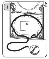
Unreel the required length of cord. It is important to keep the cord short. **Risk** of fire or electric shock. Pack the excess cord length in the cord tidy.
