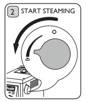
Slowly open the Valve. The steam will flow from the Nozzle and start to rotate the milk like a whirlpool. To speed up the process, gradually open Steam Valve. Take care not to splash the milk.
