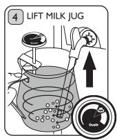
Once there is sufficient milk textured, raise the jug and continue until the Steam symbol is reached on the Thermometer Dial. CAUTION: Close the Steam Valve before removing Steam Wand from jug.
