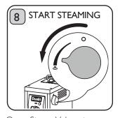
Open Steam Valve; steam will dispense initially, followed by Descaling solution. Dispense all solution. Indicator Light will flash Red and Amber when Water Tank is empty.
