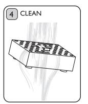
CAUTION: Allow Drip Tray to cool down before emptying. Clean Drip Tray with warm soapy water using a non-abrasive pad and dry. Wipe up any Descaler overspill.
