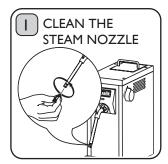
Unscrew the Steam Nozzle anti-clockwise and use a pin to remove dried milk. If too tight to unscrew, use an 8mm spanner. Screw Steam Nozzle back onto the steam wand, ensuring it is tight.
