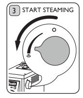
Slowly open the Steam Valve to halfway. Pump will start and steam will flow from the Steam Wand Nozzle. To speed up the process, gradually open the Steam Valve, take care not to splash milk.
