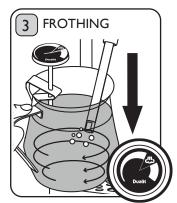
As the thermometer dial starts to rise, lower the lug to bring the Nozzle to the surface of the milk. This will start to introduce air and develop the froth. Large bubbles indicate nozzle is raised too high.
