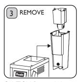
CAUTION: Remove Water Tank from machine then remove Water Filter Holder from Water Tank. Do not allow Descale Solution to come in contact with Dualit Water Filter. **Risk of injury or contamination.**
