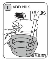
Add milk to the jug. Holding the lug by the handle, and at a slight angle, place the tip of the Steam Wand Nozzle 1-2 cm below the surface. The wand should be close to the edge of the jug, not in the centre.
