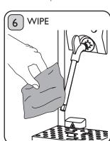
After each frothing, open the Steam Valve to clean. Immediately wipe the Steam Wand with a damp cloth. WARNING: Steam Wand will be hot. Turn the machine off using the ON/OFF switch and unplug.
