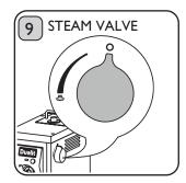
Close Steam Valve ,discard Descale solution, following the Descaler instructions. Leave for 10 minutes to allow time for the solution to take effect. Do not switch off the machine.
