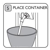
Place Water Tank back into machine. Place a container with a capacity of more than 2 litres on top of the Drip Tray, located under the Steam Wand. Ensure Drip Tray is located against the front surface of the machine.
