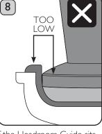
If the Headroom Guide sits below the top of the Cup Filter, there is too little coffee. Increase the grind time by I second and grind again. Keep adding I second at a time until the Headroom Guide aligns with the top of the Cup Filter.
