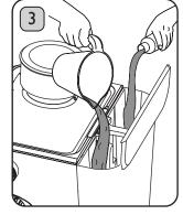
Fill the Water Tank with a minimum of 1.5 litres of water and the recommended amount of descaler (see the instructions on your descaler).
