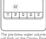
will flash on the Display Panel. Press the Espresso Button to decrease the volume by Iml per press. Press the Double Espresso Button to increase the volume by Iml per press. The volume range is 10ml to 80ml.
