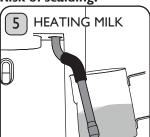
To heat the milk only, leave the Steam Wand positioned well under the surface of the milk. Do not move the Milk lug. Caution: Never allow the milk to boil. Risk of scalding.
