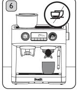
Place a cup under the Portafilter and press the Double Cup Button to dispense water through the Portafilter and clean the internal pipework. Place a cup under the Hot Water Tap and turn the Steam/Hot Water Lever to hot water position for 10 seconds. Then turn the Lever back to the "OFF" position. Repeat this twice. Discard the water in the cup and empty the Drip Tray.
