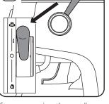
from a cold start e.g. the first use of the day/just switched on, prime the Steam Wand by turning the Steam/Hot Water Lever to the Steam position. Run steam for 3 to 5 seconds before turning to the "O" position.
