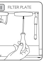
Remove the Drip Tray. Using a Philips screwdriver (PH2), remove the screw from the centre of the Filter Plate.
