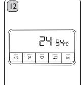
The Display will count up the extraction time and stop automatically when the dose is reached. The coffee machine is preset to extract 35ml of coffee for a single cup and 70ml for a double cup.
