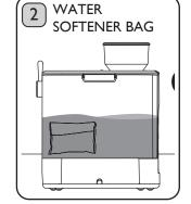
Follow the instructions provided with the Water Softening Bag to install in the Water Tank. Ensure that the Water Tank is filled with fresh water, not exceeding the "MAX" mark. DO NOT USE ANY OTHER LIQUID.
