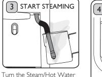
Lever to the Steam position. The Steam Indicator will illuminate, the pump will start and steam will dispense for up to 5 minutes continuously. Then the machine will beep. For best results, use a thermometer to measure the temperature of the milk while you are steaming and aim for around 67°C. Risk of scalding.
