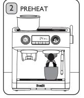
Preheat the Portafilter, Cup Filter and cup for best results. Place the required Cup Filter into the Portafilter and attach to the Group Head, turning anti-clockwise until it stops. Place your cup under the Group Head and press the Single or Double Cup Button. Water will dispense into the cup. Also, warming the Cup Filter and Portafilter provides a hotter drink and ensures they are clean and not blocked.
