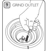
Use the Grind Outlet Brush to remove any build-up of debris in the Grind Outlet or on the Lower Burr. A torch is useful to check that the Grind Outlet is clean of loose coffee and oil build-up from the beans.
