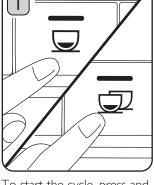
To start the cycle, press and hold the Esprésso or Double Espresso Button depending on which you would like to adjust, until the appliance beeps once and the selected button flashes. You can now adjust the settings.
