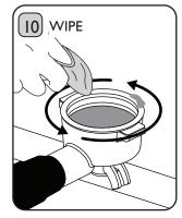
Remove the Tamper and clean any excess coffee grounds from the rim of the Cup Filter. .....
