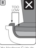
If the Headroom Guide sits below the top of the Cup Filter, there is too little coffee. Increase the grind time by I second and grind again. Keep adding I second at a time until the Headroom Guide aligns with the top of the Cup Filter.
