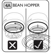
Ensure the bottom of the Bean Hopper is correctly aligned before attempting to attach the Bean Hopper to the machine. If it is not correctly aligned, push the Tab in the direction shown until it is in the correct position. 4B GRIND INLET
