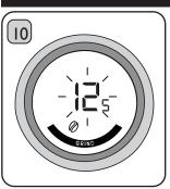
Press and hold the Grind Button until the appliance beeps and the time shown on the Grind Screen flashes. Press the Espresso Button to decrease the time by I second per press. Press the Double Espresso Button to increase the time by I second per press. The grind time range is 1 to 60 seconds.
