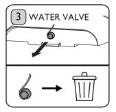
Remove the red seal from the Water Valve by pulling the tab and check there is no other packaging inside. Replace the Water Tank.
