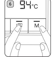
Press the Power Button to switch the appliance on. Press and hold the Double Cup and Manual Buttons at the same time until the appliance beeps once.
