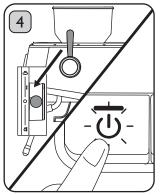
Ensure that the Steam/ Hot Water Lever is in the "OFF" position. Plug in the Power Cord and press the Power Button. The Grind Button will illuminate. The Power Button and Function Indicator will flash for up to I minute to indicate you're in Preheat mode.
