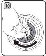
With the Upper Burr Handle aligned parallel to the front of the coffee machine, slowly rotate clockwise until the Upper Burr drops down. Then, using the Upper Burr Handle, rotate clockwise until it clicks into place and the handle is parallel to the side of the coffee machine. There are markings to indicate which way to turn the Upper Burr into place.
