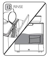
Thoroughly rinse the Water Tank and fill with fresh water. Repeat steps 6 to 11 with water only to remove any trace of descaling solution. Replace the Water Softening Bag and refill the Water Tank with fresh water.
