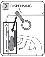
Turn the Steam/Hot Water Lever to the Hot Water position. The Hot Water Indicator will illuminate and hot water will dispense. Note: The Hot Water Tap will not operate whilst coffee is extracting. Risk of scalding.
