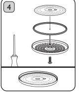
Place the O-Ring into the Large Filter Plate, then place the Small Filter Plate as shown. Position the assembled Plates back into the Group Head, rethread the screw and tighten.
