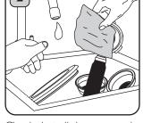
Check that all the accessories and attachments are complete and not damaged. Ensure that the machine is unplugged. Wash the Hopper Lid, Water Tank, Drip Tray, Portafilter and Cup Filters in warm, soapy water. Rinse and dry thoroughly. Wipe the Bean Hopper with a damp cloth. WARNING: Do not submerge the Bean Hopper. Dry thoroughly.
