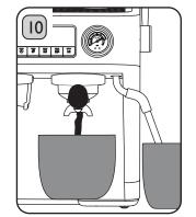
Turn the Steam/Hot Water Lever to the Hot Water position. The Hot Water Indicator will illuminate and water will dispense from the Hot Water Tap. This will take approximately 2 minutes and dispense around 500ml water.
