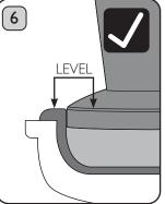
**Pro's Tip:** Use the Tamper as a guide to check you have the correct amount of coffee. The top of the Tamper should be level with the top of the Cup Filter. For more detail on tamping, see page 18.
