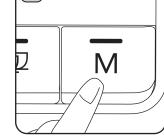
Press the Manual Dosing Button once to confirm the grind time. The appliance will beep once.
