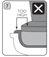
If the Tamper is sitting too high, there is too much coffee. Reduce the grind time by I second and grind again (see page 21). Lower by I second at a time until the Headroom Guide aligns with top of the Cup Filter. See page 23 for how to adjust presets.
