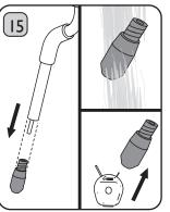
Ensure that the Steam Wand is cool before cleaning. Using your fingers, unscrew the Froth Nozzle from the Steam Wand, wash under running water to remove any milk residue. Using the thinner Cleaning Pin, remove dried milk from the Frothing Nozzle. **Risk** of burns. WARNING: Cleaning Pin is sharp, take care when cleaning. **Risk of** injury to persons.
