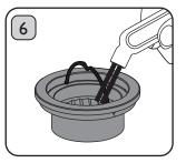
Use the Cleaning Bush to remove any coffee from the Upper Burr. Do not immerse the Upper Burr in water. Remove stubbom coffee build-up with a damp cloth and dry thoroughly. WARNING: Burrs will have sharp edges, take care when cleaning. **Risk of injury to persons.**
