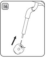
Use the thicker Cleaning Pin to remove dried milk from the Steam Tube. WARNING: Cleaning Pin is sharp, take care when cleaning. **Risk of injury to persons.**
