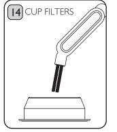
Use the Cleaning Brush to remove any coffee build-up on the Cup Filters.
