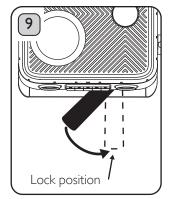
When you are happy with the coffee grounds in the Portafilter, attach to the Group Head and rotate Portafilter anti-clockwise to lock into place. Press the Double Cup Button.
