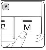
Press the Manual Dosing Button once to confirm the extraction water volume. The appliance will beep once. You have now completed the cycle and the appliance is ready to use.
