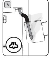
Once Preheating is complete, the appliance will enter Standby mode (indicated by all buttons illuminating) and is ready to use. Position the Steam Wand in the Milk Jug. Turn the Steam/Hot Water Lever to the Steam position and run steam through the Steam Wand for 10 seconds.
