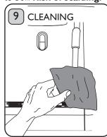
After every use, flush the Steam Wand by dispensing steam to remove milk residue from inside the Steam Wand. Wipe the Steam Wand with a damp cloth. **PRODUCT** FAILURE DUE TO THE BUILD-UP OF **MILK RESIDUE IS NOT COVERED BY YOUR GUARANTEE.** Keep hands away from steam and Steam Wand.
