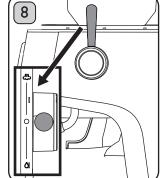
To stop steaming/frothing turn the Steam/Hot Water Lever to the "O" position. Ensure steaming has stopped before removing the Steam Wand from the Milk Jug. Risk of scalding.
