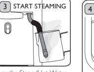
Turn the Steam/Hot Water Lever to the Steam position. The Steam Indicator will illuminate, the pump will start and steam will dispense for up to 5 minutes continuously. Then the machine will beep. For best results, use a thermometer to measure the temperature of the milk while you are steaming and aim for around 67°C. Risk of scalding.
