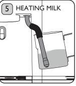
To heat the milk only, leave the Steam Wand positioned well under the surface of the milk. Do not move the Milk lug. Caution: Never allow the milk to boil. Risk of scalding.
