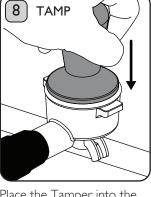
Place the Tamper into the Cup Filter, gently pressing downwards. Stop when the Headroom Guide is level with the top of the Cup Filter.
