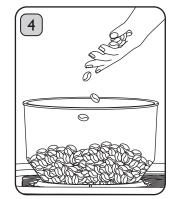
Top up the Bean Hopper with fresh beans if required and secure the Lid. Remember to only grind what you need. Note: Check your coffee beans for foreign objects e.g. glass, nails or stones. **Risk** of damage and injury.
