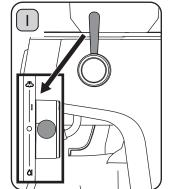
Check that the Steam/Hot Water Lever is in the "O" position.
