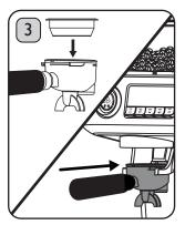
Fit the Double Cup Filter into the Portafilter and place into the Portafilter Cradle. Press the Grind Button once. Press again to stop grinding, if ground coffee has formed a high mound and is overflowing. Note the time this took.
