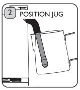
Pour cold milk into the Milk Jug until it is half-full. Hold the Milk lug by the handle and tilt at a slight angle. Position the Frothing Nozzle (at the end of the Steam Wand) just under the surface of the milk, ensuring it is fully submerged to prevent milk splashback. **Risk of scalding.**
