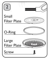
Remove the two Filter Plates and O-ring. Using the Cleaning Brush, remove any build-up of coffee grounds. If required, wash in warm, soapy water and dry thoroughly.
