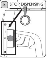
Once the Power Light flashes and the machine beeps twice, turn the Steam/ Hot Water Lever to the "O" position to stop the water flow.
