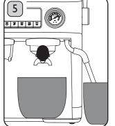
Place a plastic container with a 1.5 litre capacity under the Group Head and another under the Steam Wand.
