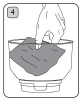
Wipe the Bean Hopper clean with a damp cloth, then dry thoroughly before storing. WARNING: do not submerge Bean Hopper in water, as water will get trapped in valve mechanism.
