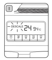
The Descale Indicator will be flashing to warn a descale is due, or illuminated solidly to indicate the appliance is in lockdown and will not operate.
