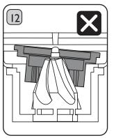
If the Hopper does not fit, lift it off and check that the Upper Burr is in the correct position - adjust and re-fit Hopper.
