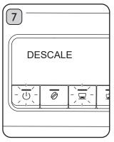
The Power Button will illuminate and the Single Cup Button will flash. You have activated the Descale programme.
