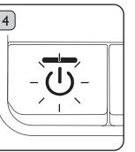
After 5 minutes, the machine will beep twice, the Power Button will flash and the Steam Wand will stop dispensing. For more steam, turn the Lever to the "O" position and then turn back to the Steam position. **Risk** of scalding.
