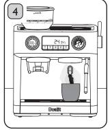
The Hot Water Tap will dispense up to 200ml at one time. For more hot water, turn the Lever to the "O" position and then turn back to the Hot Water position. **Risk of scalding.**
