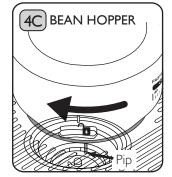
Check that there are no foreign bodies in the Bean Hopper. Fit the Bean Hopper into position by aligning the unlock symbol with the Pip at the front, gently pressing the Bean Hopper down and rotating clockwise. Do not force the Bean Hopper if it feels tight when turning. If it does feel tight, remove the Bean Hopper and repeat steps 4A to 4C. **Risk of damage to the machine.**
