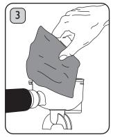
Discard the water from the cup. Remove the Portafilter from the Group Head and dry the inside of the Cup Filter with a cloth. Caution: Portafilter will be hot. Always hold by the handle, do not touch the metal Cup Filter. **Risk of burns and** scalding.
