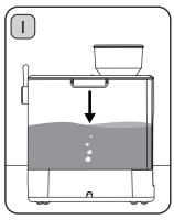
Fill the Water Tank with fresh water; do not go above the "MAX" mark. You will see air bubbles at the connection when correctly located. Plug in the Power Cord and press the Power Button once. The appliance will beep once and the Display will illuminate. Avoid letting the Water Tank run empty.
