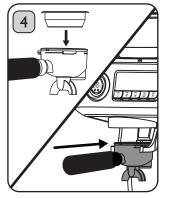
Fit the 2 Cup Filter to the Portafilter, empty of coffee. Attach to the Group Head. DO NOT SOAK THE PORTAFILTER OR FILTER CUPS IN DESCALING SOLUTION. Ensure they are rinsed thoroughly after descaling.
