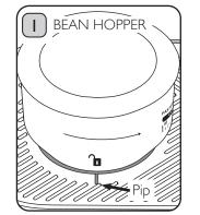
Clean the Grinding System once a month or before changing coffee beans, to avoid flavour tainting. Rotate the Bean Hopper anticlockwise until the unlock symbol meets the Pip. Lift to remove the Bean Hopper and empty any beans into an airtight container to store.
