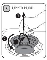
Lift up the Upper Burr Handle (1) and use it to turn the Upper Burr anticlockwise until you hear a click (2). Lift out the Upper Burr (3). 29
