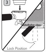
Insert the Double Cup Filter into the Portafilter (ensure Cup Filter is empty of coffee). Attach the Portafilter to the Group Head and rotate anticlockwise until resistance is felt.
