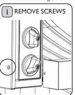
Remove the two screws seen on the left and right-hand sides of the controls. Align the Anti-Tamper Guard with the screw holes.
