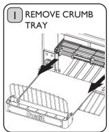
Remove the Crumb Tray. From a cold start, set the Conveyor Toaster to standby. Select toast setting 9. As the conveyor rotates, clean the exposed section of the belt. Wipe with a damp, non-abrasive cloth if lightly soiled or a dry, lightly abrasive pad if heavily soiled. Then wipe with a damp cloth.
