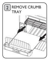
Turn off and unplug the toaster. Remove the Crumb Tray and lay the toaster on its right hand side, onto a cloth to protect the surfaces, to gain access to the reset button. Warning: Take care not to pull or knock the legs when turning the product over. Damage may occur.
