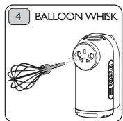
The Balloon Whisk can fit into either hole. Grasp the handle of the Mixer with one hand and the Balloon Whisk stem with the other hand. Insert the Balloon Whisk with a slight twist and push action until it clicks into place.
