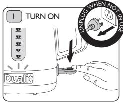
Plug the kettle into the power socket. Press the 'On/Off' switch down. The power neon will illuminate and the kettle will start to heat up. If the kettle is accidentally switched on with no water inside, the boil-dry device will switch off the Always unplug the kettle after each heating element to prevent damage to the kettle. use.
