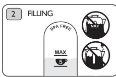
Fill the kettle through the lid opening. Use at least one cup of water (250ml). The water level must stay below the 'max' mark. Save energy, only boil what you require. Keep kettle uprigh and level at all times when filling (maximum 15° incline). Do not tilt kettle backwards. DO NOT JUST BOILED, THE METAL PARTS **OVERFILL OR FILL THROUGH THE**
