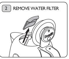
Unplug and let the kettle cool. Open the lid. Hold the top of the filter, pull up and out of the kettle. Rinse under a tap while carefully brushing it with a soft brush. Rinse the kettle out with fresh water. **DO NOT OPERATE**
