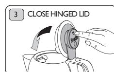
Push the lid down until it clicks. Check that it is fully in place, otherwise the kettle may not switch off when boiling.
