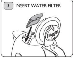
Ensure water filter is in place. **DO NOT OPERATE KETTLE UNLESS THE** WATER FILTER IS CORRECTLY IN POSITION.
