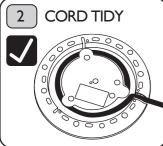
Use the shortest cord possible. cord tidy on the base of the kettle.
