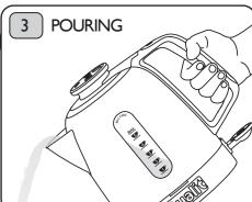
Remove kettle from the power base. When filling or carrying the kettle, do not tilt it backwards, as this may allow water to pass through the steam tube onto the control area. Should this happen, the kettle must be allowed to dry before re-using. To avoid the risk of splashing, once the kettle has boiled wait 10 seconds then pour slowly. Do not over-tilt the kettle.
