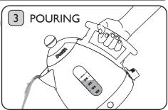
Remove kettle from the Power Base. When filling or carrying the kettle, do not tilt it backwards, as this may allow water to pass through the Steam Tube onto the control area. Should this happen, the kettle must be allowed to dry before re-using. To avoid the risk of splashing, once the kettle has boiled wait 10 seconds then pour slowly. Do not over-tilt the kettle.
