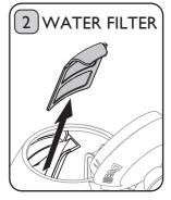
Make sure the appliance is switched off, unplugged and allowed to cool. Open the Lid. Hold the top of the Water Filter, pull up and out of the kettle. Rinse under a tap whilst brushing carefully with a soft brush. Rinse out the kettle with fresh water. To replace align the Water Filter with the grooves in the Filter Holder, insert and push back into place. Do not operate kettle unless water filter is correctly in position. Risk of scalding and injury caused by misuse.
