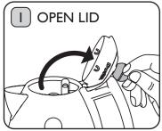
Ensure the kettle is unplugged. Remove the kettle from the Power Base. Pull the Knob up and towards the Handle to open the Lid. The Lid is Pushing the Lid Pips back out will hinged for easy opening and closing. WARNING: IF THE KETTLE HAS JUST BOILED, THE LID WILL BE HOT. USE THE KNOB TO CLOSE THE LID.
