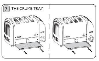
Crumbs will accumulate in the crumb tray and could catch fire if the tray is not emptied frequently. Pull out the crumb tray and wipe clean using a damp cloth. CRUMB TRAY MUST BE IN PLACE BEFORE TURNING ON THE TOASTER AND DURING TOASTING.
