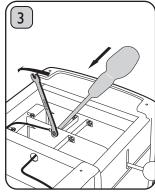
Unscrew brass links and wires.
