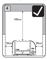
Place the toaster on an open level surface. Ensure the toaster is positioned at least
