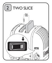
**2, 3 & 4 slot model:** Select the two slice indicator. The two slots from the left will toast on both sides.
