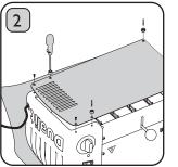
Remove the crumb tray and toaster base plate to access the fuse.
