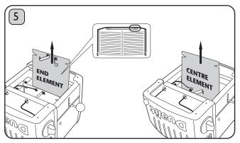
Remove element. To reassemble, reverse procedure ensuring wires and parts are correctly positioned. Ensure new element is marked the same as the one removed. The element heats on both sides and can be inserted facing either way. Check it is seated correctly in the channels either side. Portable Appliance Tested before use.
