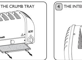
Crumbs will accumulate in the crumb tray and could catch fire if the tray is not emptied frequently. Pull out the crumb tray and wipe clean using a damp cloth. Take care when cleaning. **CRUMB TRAY MUST BE IN PLACE**
